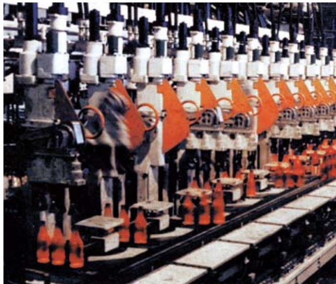
Controlling Shock Loads On Independent Station Glass Molding Machines...
